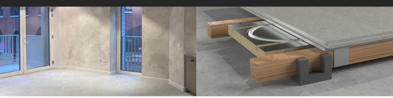
For the 120 marketed apartments we installed EDB underfloor heating with our acoustic cradle and batten system, topped with18mm GIFA board. This provided a stable substrate for the large format 600mm x 1200mm marble floor tiles, and would also ensure the efficient transfer of heat.
